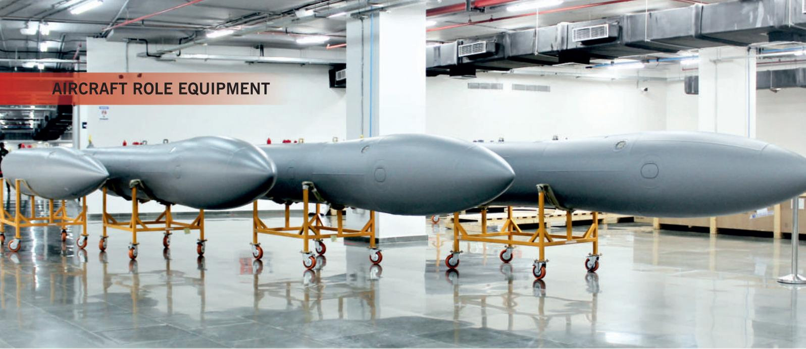
Defsys is the indigenous manufacturer of aircraft Role Equipment, a Build to Print production transfer program with an International OEM. The Role Equipment include Pylons, Fuel Tanks and Bomb Racks. The scope of the project encompasses complete manufacturing, assembly, integration and testing of the Role equipment which are currently being manufactured. Defsys has delivered hundreds of items of Role Equipment with a 100 percent defect free record.
